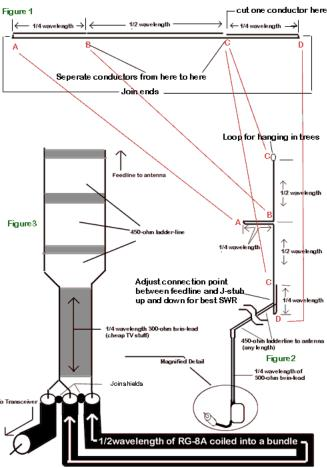
Don't forget to calculate the velocity factors of the transmission and phasing lines
